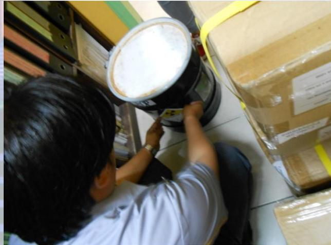
**16.** Affix a leaded tamper proof safety seal onto the shipping drum locking ring and fasten with a hammer or other suitable means.
